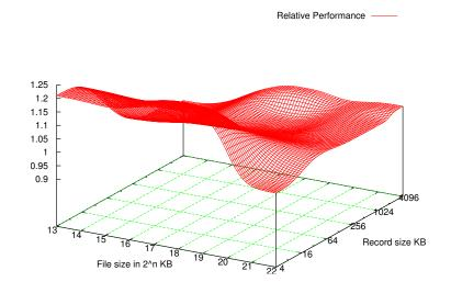
Figure 5.4: TxBtrfs's relative performance to Btrfs's, for Write operations
