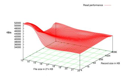
Figure 5.1: TxBtrfs's Throughput for Read operations
