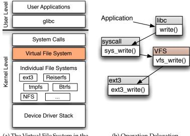
(a) The Virtual File System in the System Stack
