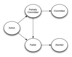
Figure 2.4: A Transaction's State Diagram (taken from [SKS06])
