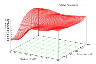
Figure 5.2: TxBtrfs's relative performance to Btrfs's, for Read operations
