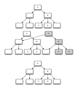
Figure 2.3: Copy-On-Write on Btrfs.
