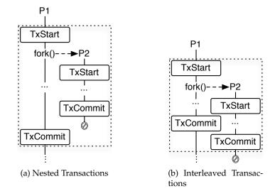
Figure 4.2: Different scopes for inner-transactions
