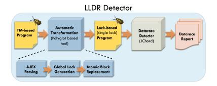
Fig. 2. The low-level datarace detection procedure.
