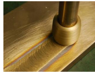
Friction Stir Surfacing
