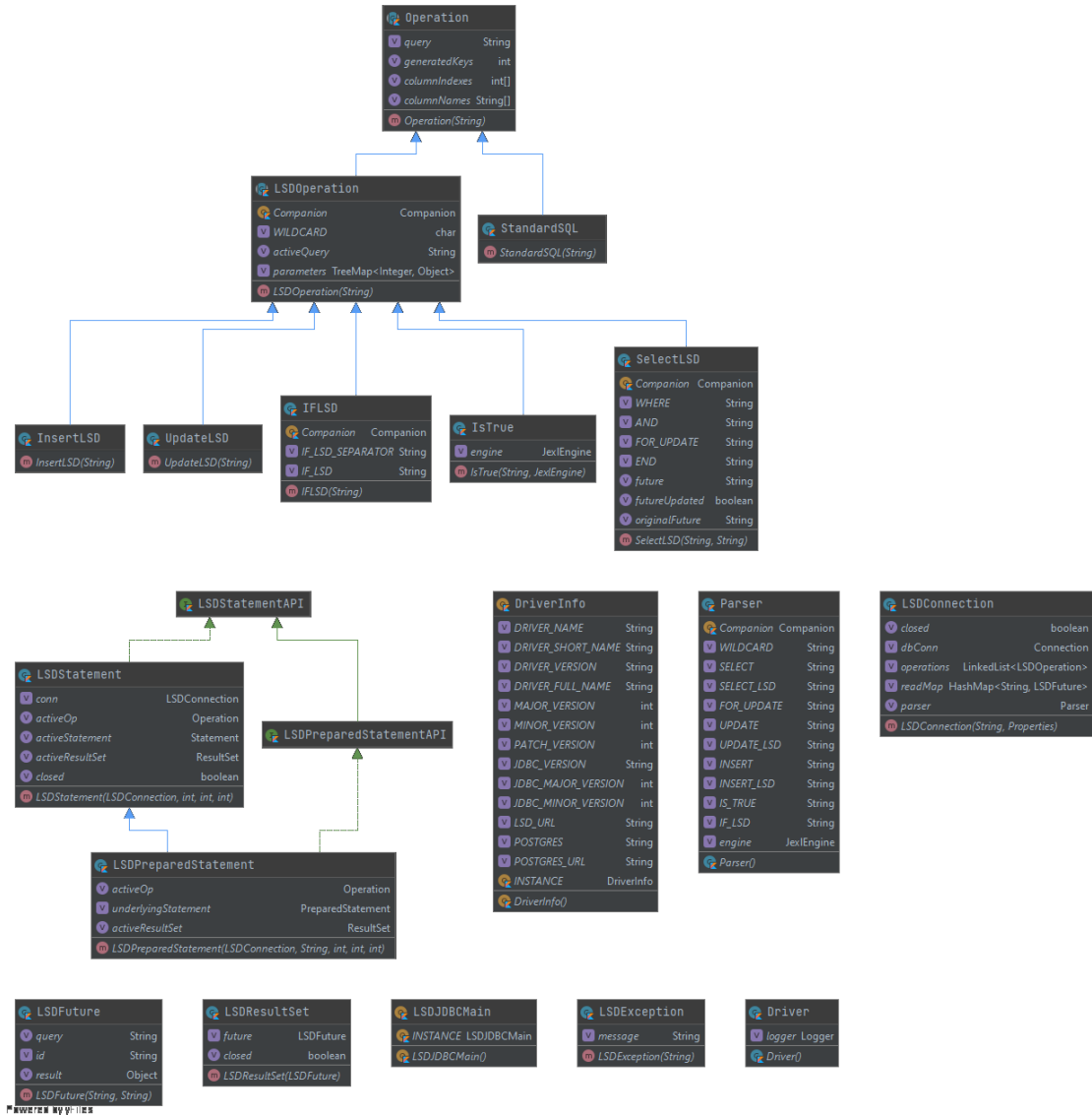
Figure A.1: LSD-JDBC Driver Detailed Class Diagram, made with IntelliJ IDEA's UML plugin[44]
