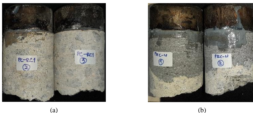
Figure 91. Pull-off test cores: (a) PC-RC1; and (b) PRC-U.
