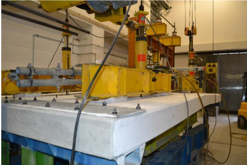
Figure 8 – Photo taken during the test of specimen C-HP960-L during a 6% drift cycle
