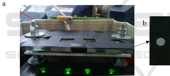
Figure 4: (a) Opaque masks layers implemented to prevent the interference of dispersed light from the LEDs in the surroundings with the LDRs response. (b) Sensing film with an opaque mask applied.
