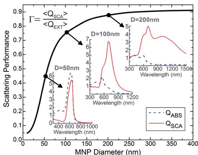
Fig. 2 Scattering performance ( $\Gamma$ ) of single spherical Au NPs immersed in a AZO medium, evaluated along the 300–2000 nm spectral range, as a function of the NPs diameter. The insets show the  $Q_{\text{SCA}}$  and  $Q_{\text{ABS}}$  of particles with 50, 100 and 200 nm diameter ( $D$ ). The quantities were computed with an analytical Mie theory formalism.<sup>31</sup>
