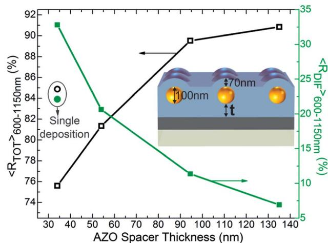
Fig. 6 Average  $R_{\text{TOT}}$  (open symbols) and  $R_{\text{DIF}}$  (filled symbols), along the 600–1150 nm wavelength range, for PBRs with distinct AZO spacer thickness ( $t$ ). The structure of the PBRs is sketched in the inset and its MNP array is composed of a double deposition of  $D = 100$  nm Au colloids. The two circular symbols at  $t = 35$  nm show the average  $R_{\text{TOT}}$  and  $R_{\text{DIF}}$  of a PBR with the same structure but with only a single deposition of MNPs.
