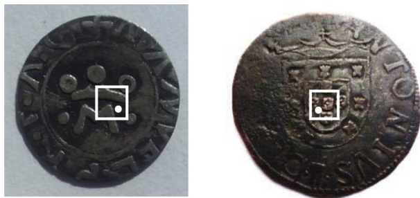
Fig. 1. Photos of studied coins. Left panel: Reverse of the 5 Reais silver-copper coin minted during king Manuel I reign (1495–1521). Right panel: Obverse of the 2 Reais copper coin minted during D. António regency (1580–1583). The squares indicate the areas covered by the 2D PIXE maps (scan 2640 \times 2640 \mu\text{m}^2 ); The dots indicate the locations of PIXE + EBS point analysis ( 3 \times 4 \mu\text{m}^2 ).
