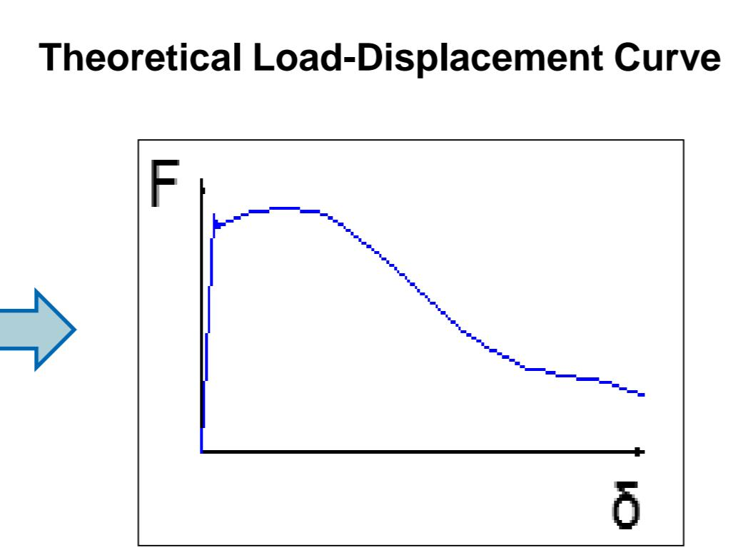
Apply inverse analysis to compute  $\sigma$ - $w$  parameters that minimize the error,  $\varepsilon$ , between the Load-Displacement curves
