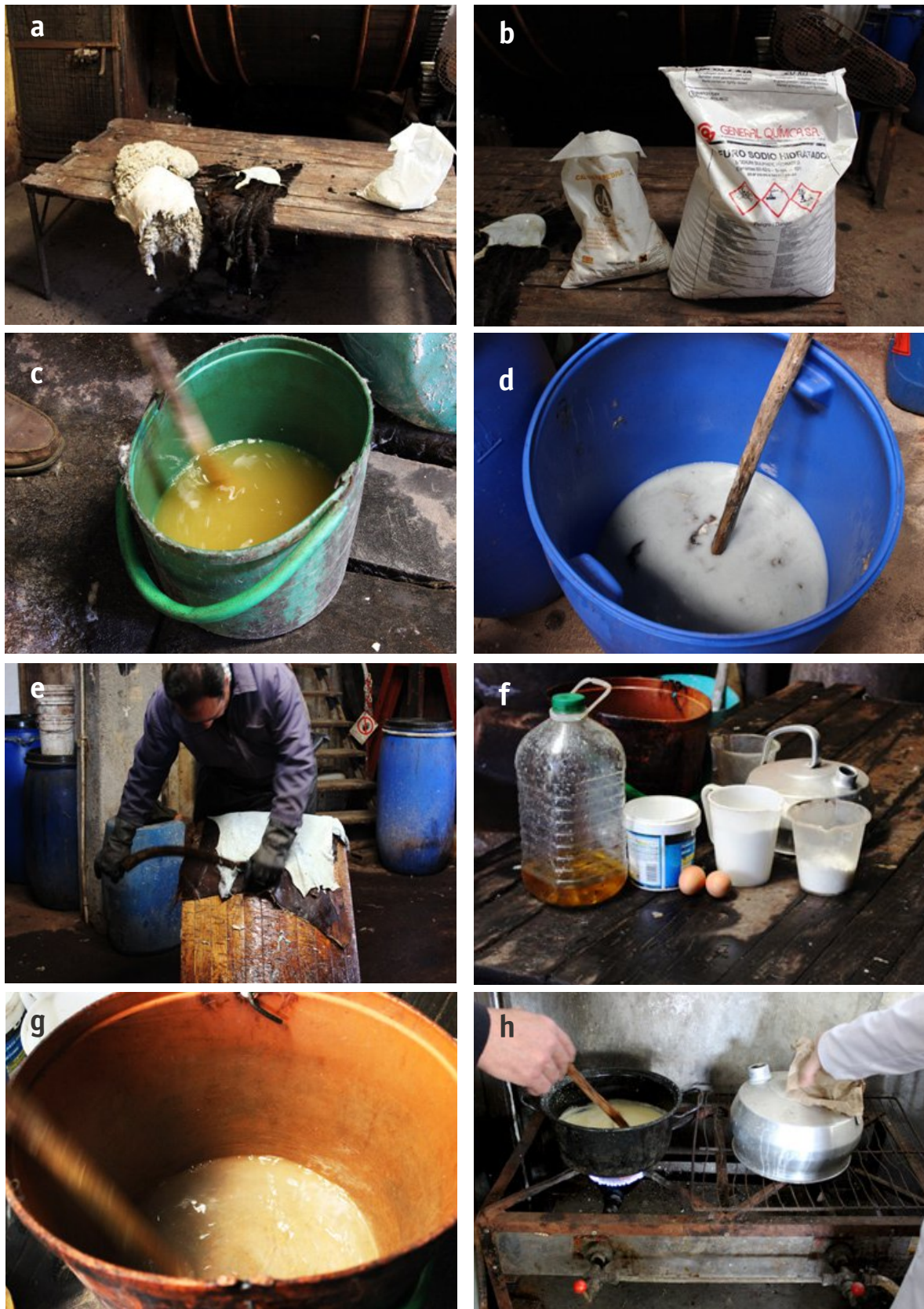
Figure 7. Main steps of the thawing procedure of two animal skins: a) sheep (white) and goat (black) skins; b) chemical reagents used for depilating the skins (sodium sulphide ( \text{Na}_2\text{S} ) and calcium hydroxide, \text{Ca}(\text{OH})_2 ); c) preparation of the mixture for the depilation; d) immersion of the skins into the mixture; e) mechanical removal of the hair; f) ingredients of the Bolognese manuscript recipe; g) mixing the products for the thawing process; and h) heating the mixture before the treatment of the skins..
