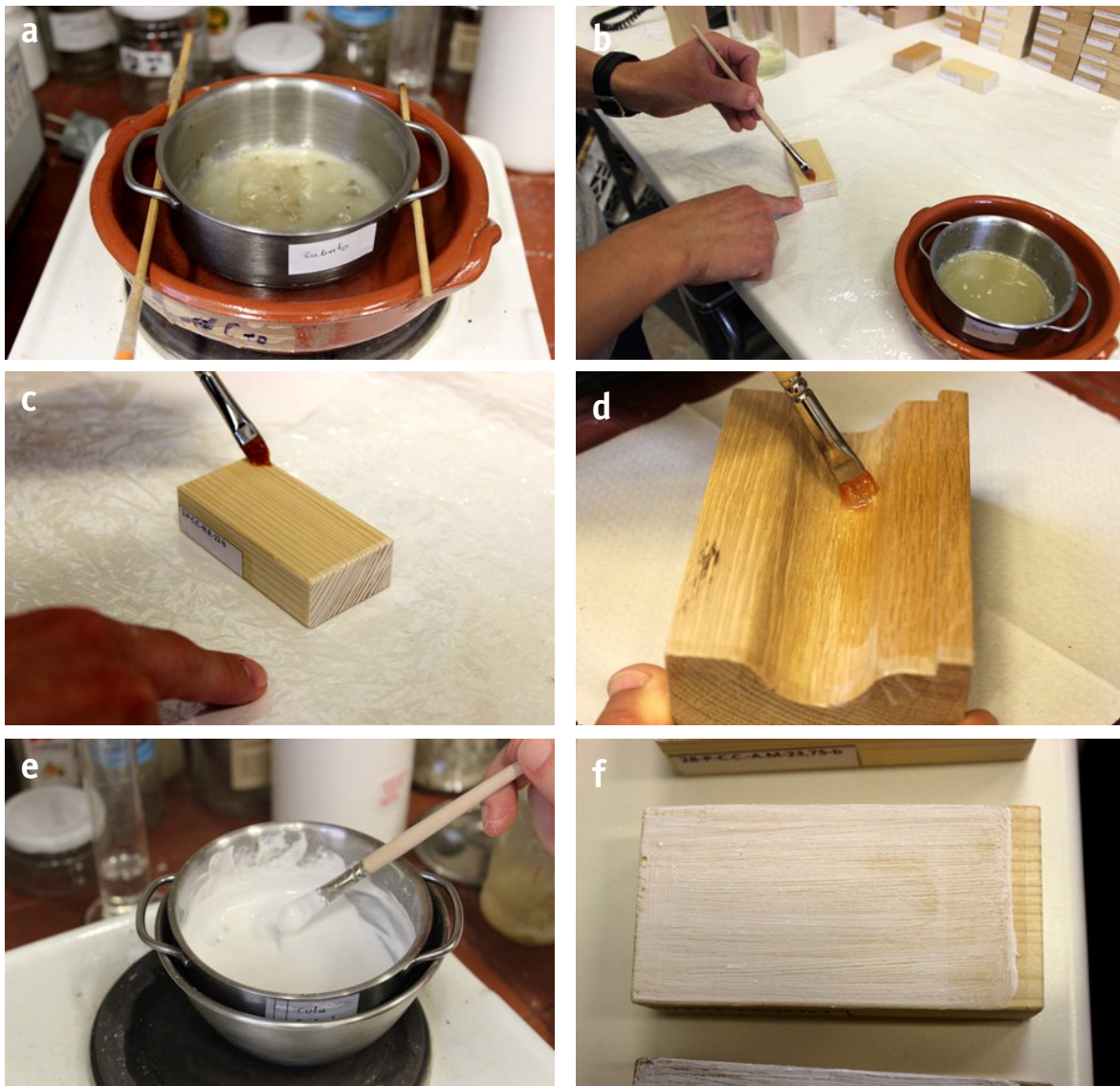
Figure 10. Main steps to the application of ground layers: a) Heating in “warm water bath” the goat gelatine; b) keeping the gelatine solution warm; c) first application of animal size with brush in flat sample; d) first application of animal size with brush in three-dimensional sample; e) mixing gesso with the gelatine; and f) application of first layer of ground on the flat sample.
