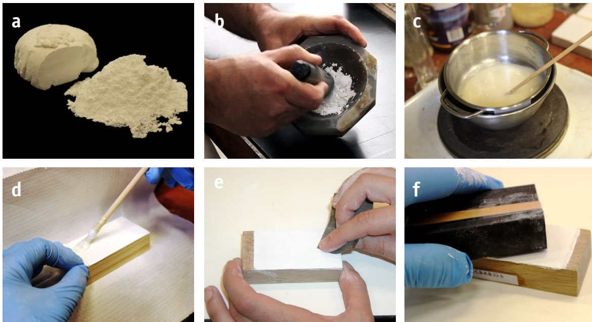
Figure 12. Main steps to prepare ground and its application: a) sieving the loaf of gesso; b) grind the gesso in mortar to obtain gesso fine powder; c) mixing it with animal glue solution in a “warm water bath”; d) application with brush of several gesso fino layers; e) sanding the surface with an abrasive paper; and f) final sanding with fine abrasive paper.
