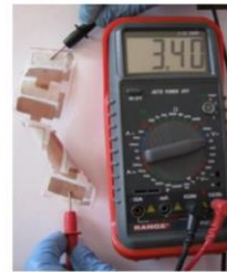
cellulose -paper battery concept
