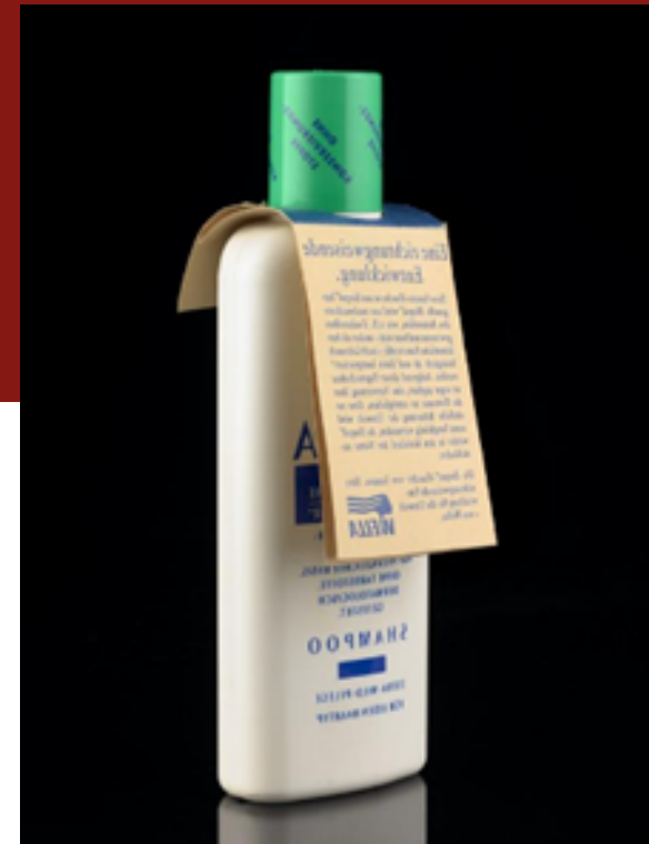
Sanara shampoo bottle: the first commercial application of Biopol, c.1990 © The Board of Trustees of the Science Museum
