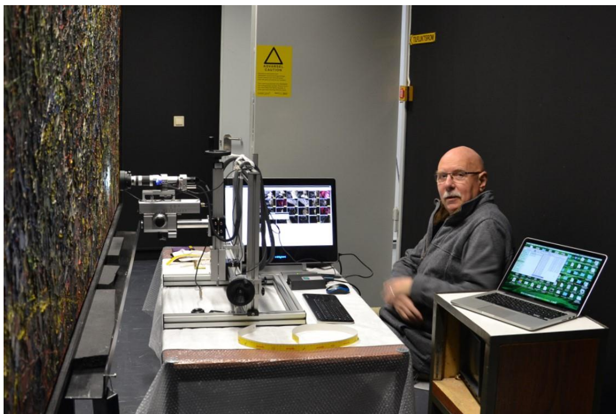
Dr Jaap Boon with the HIROX ultra high resolution microscope investigating paint defects
