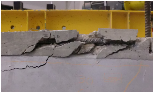
Figure 5.28: Failure in overlay concrete progressing both in a crack along the interface and a crack under the interface (beam III.B)
