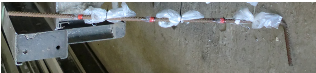
Figure 4.6: Instrumented L-shape rebar (used in SMI III)
