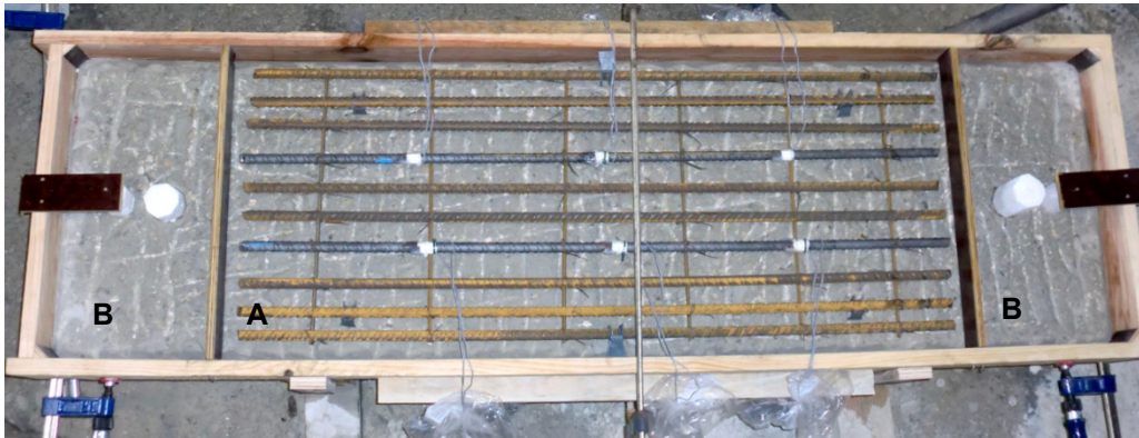
Figure 4.15: Reinforcement in the concrete overlay (SM I)
