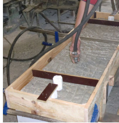
Figure 4.14: Cleaning the interface surface with compressed air
