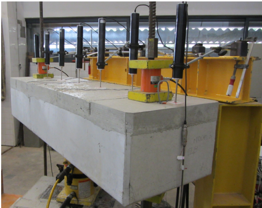
Figure 4.22: Flexural test setup
