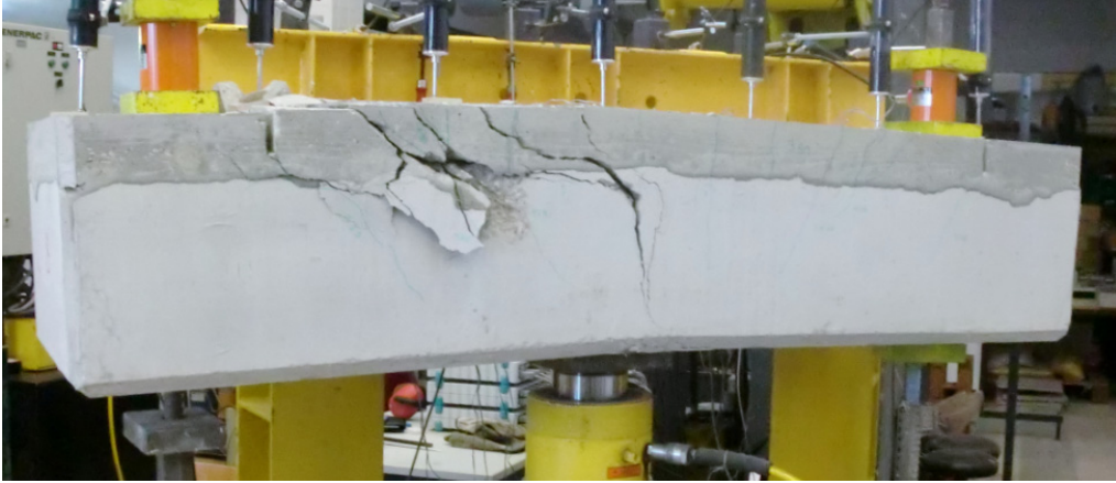
Figure 5.29: Failure mode for beam III C
