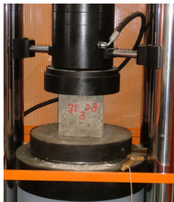
Figure 4.33: Concrete compression test
