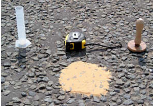
Figure 3.25: Sand patch test
