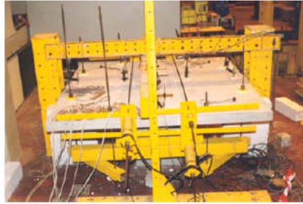
Fig. 2 System used to apply the in-plane force in slabs
