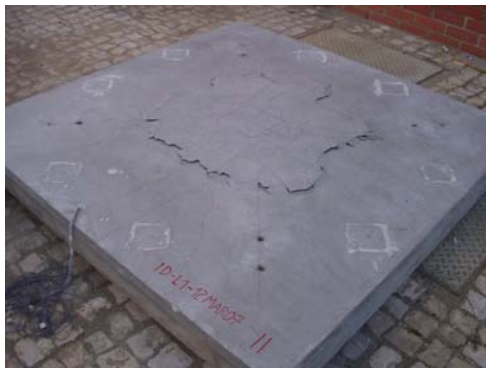
Figure 4 : Top and Bottom surface of Model ID1 after punching failure
