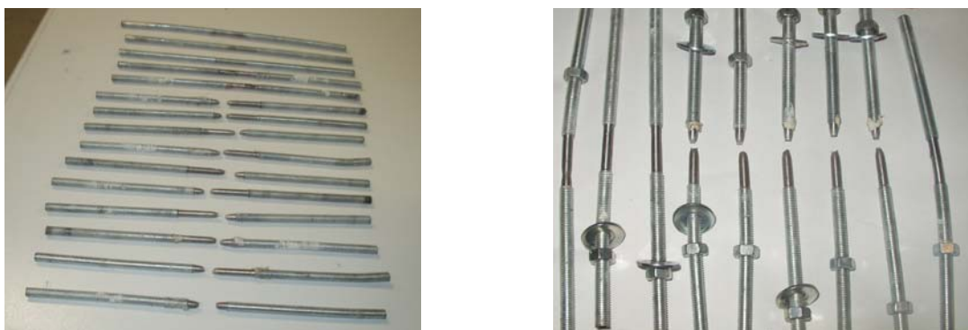
Figure 6 : Bolts after punching failure in Models ID3 and ID5
