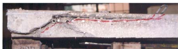
Figure 9 – Tendon location and punching shear failure surface
