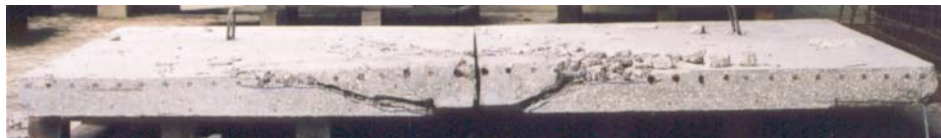
Figure 4 – Angle between the punching failure surface and the horizontal in Model AR2
