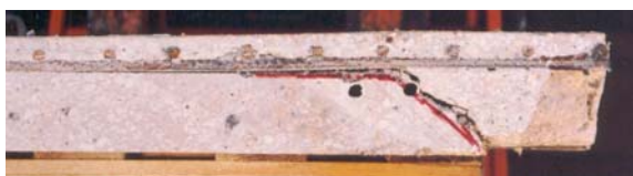
Figure 9 – Tendon location and punching shear failure surface
